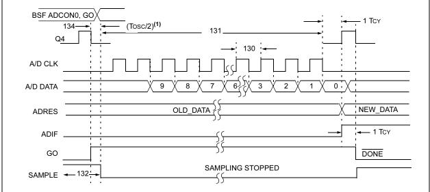
**Note 1:** If the A/D clock source is selected as RC, a time of Tcy is added before the A/D clock starts. This allows the SLEEP instruction to be executed.
