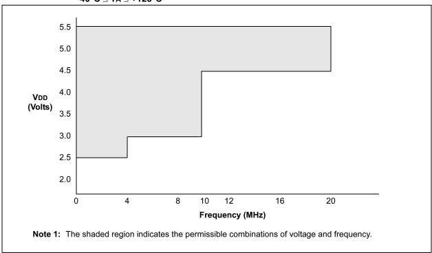
FIGURE 12-3: PIC16F676 WITH A/D ENABLED VOLTAGE-FREQUENCY GRAPH,  $0^{\circ}C \le TA \le +125^{\circ}C$
