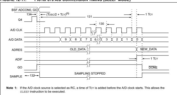
FIGURE 12-11: PIC16F676 A/D CONVERSION TIMING (SLEEP MODE)
